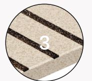
GROOVE WITH EPOXY FILLING
